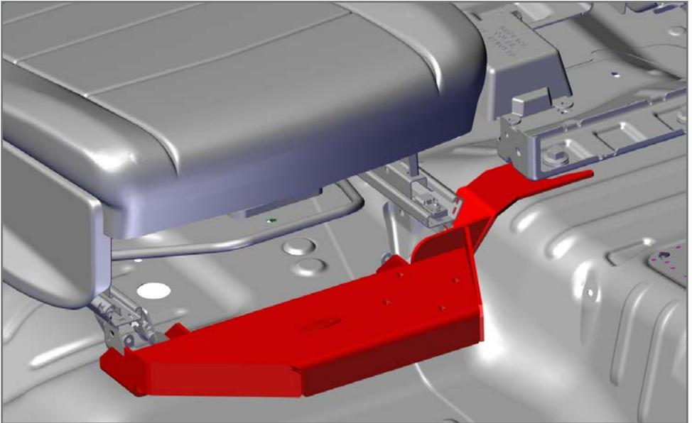
4. Replace the passenger seat back into the vehicle and place the base under the previously removed two front seat bolt locations. Wedge the tab of the HD Base support under the mounting frame of the front middle seat frame and replace previously removed OEM seat bolts securing base in place.
