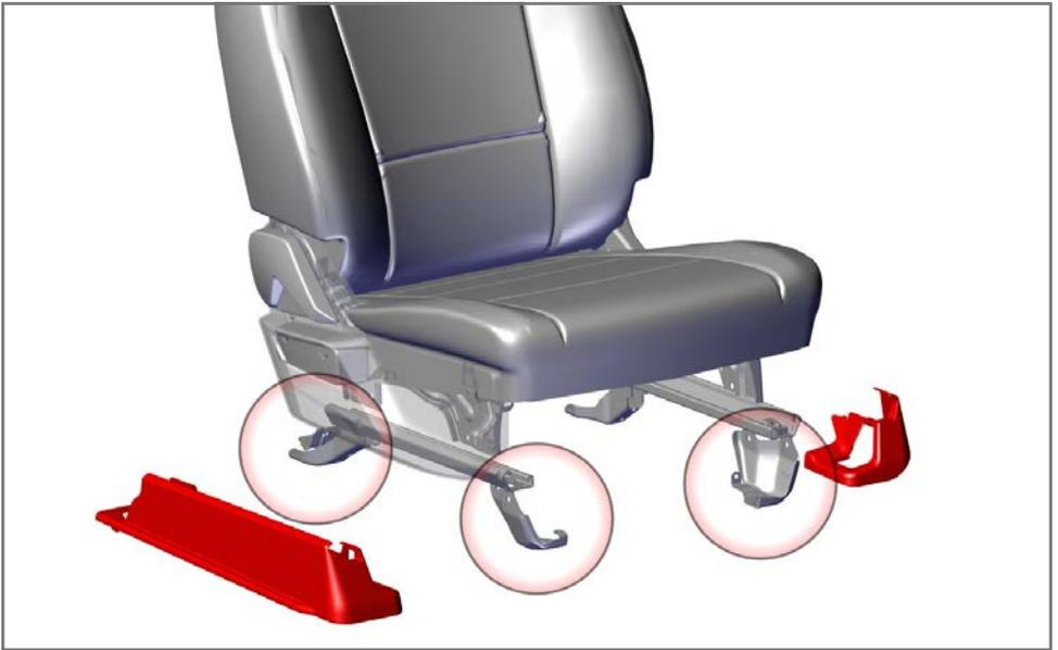
3. Remove the screws and push pin clips on the passenger's seat trim located on door side and front mounting position of the seat. **Note:** Trim not reused.
