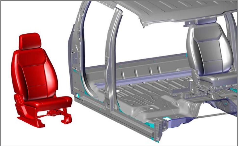
2. Remove the front and rear OEM seat bolts. Tilt the seat back and unplug any electrical connection attaching to the seat. Remove seat from the vehicle.
