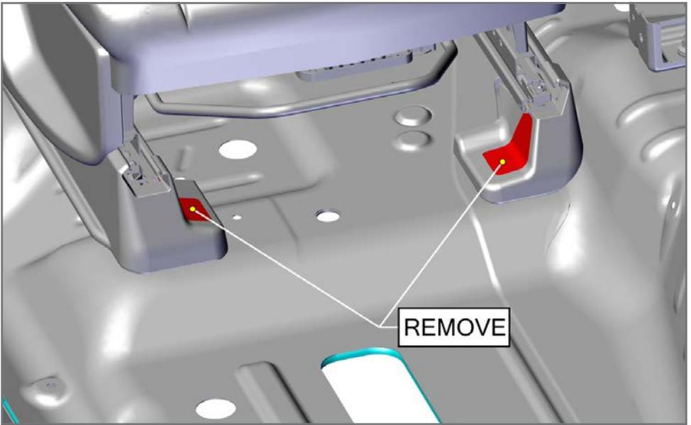
1. Remove the front and rear trim bolt covers using a small flat head screw-driver.
