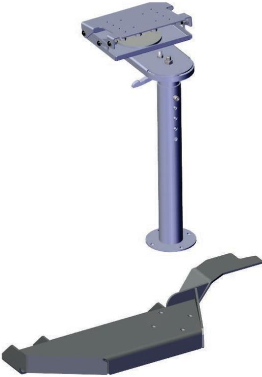
5. Use a 1/2" socket to secure the upright stand assembly to the base with the provided (4) 5/16-18 bolts and washers. **Note:** *The height adjustment bolts should be positioned bumper to bumper when properly installed.*
