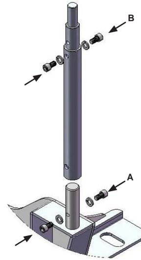
1. Remove Hex Head Cap Screws from stand assembly and place tube over the No-Holes Mount Base.
