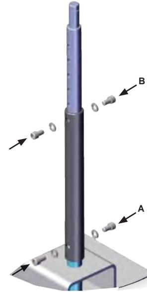
1. Remove Hex Head Cap Screws from stand assembly and place tube over the No-Holes Mount Base.
