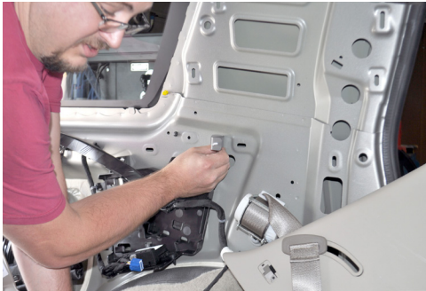
Once finished with AVK, install D/S Inner Mount Bracket.
