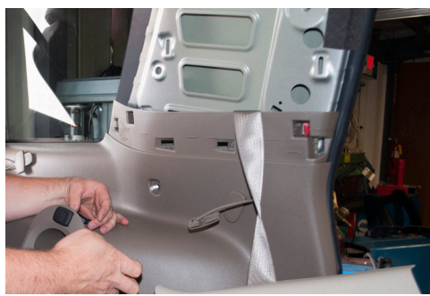
Reinstall lower OEM trim piece with Inner Mount Bracket stud sticking through drilled hole of trim.
