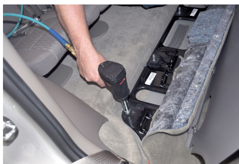
Flip second row seating up towards front seats, then flip carpet/rubber mat to expose (4) OEM nuts. Remove the (2) outer nuts using an 18 mm Socket.
