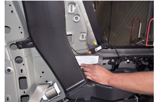
Use provided template, mark AVK hole location. Install AVK using directions on back page.
