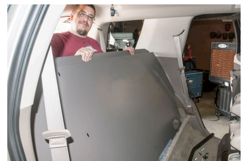
Install Lower Steel Barrier into vehicle.
