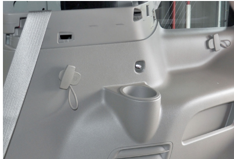
Reinstall lower OEM trim piece with Inner Mount Bracket stud sticking through drilled hole of trim.
